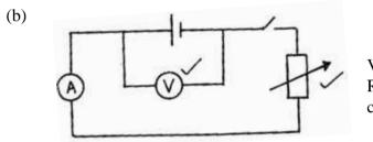
Voltmeter across cell Rheostat for adjusting current.
