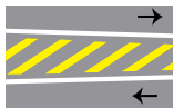
Channelizing island (do not drive over the marking except in an emergency)
