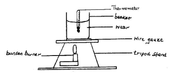
(a) Measure 100cm³ of water and pour it into the beaker. Take the initial temperature of the water.
