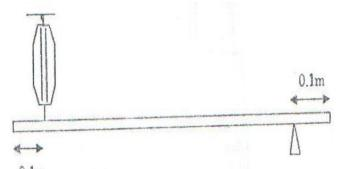
Given that the reading of the spring balance 0.6N, determine the reaction on the pivot. (3 mks)
