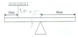
Given that the tension T in the string is 0.8N, determine the reaction force at the pivot. (3 mks)
