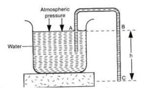
Pressure on the surface of the liquid is atmospheric pressure. Since end C of the tube is below the surface A by height h, pressure at C is greater than that at the surface.
