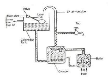
The hot water tap and expansion pipe are connected to the upper region of the cylinder. The expansion pipe is an outlet for excess water that could have resulted from overheating.
