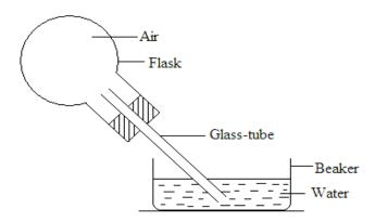
Invert the flask with glass tube dipped into the water as shown.
