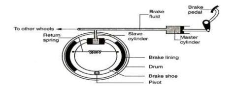
The force applied on the foot pedal exerts pressure on the master cylinder. The pressure is transmitted by the brake fluid to the slave cylinder. This causes the pistons of the slave cylinder to open the brake shoe and hence the brake lining presses the drum. The rotation of the wheel is thus resisted. When the force on the foot pedal is withdrawn the return spring pulls back the brake shoe which then pushes the slave cylinder piston back.
