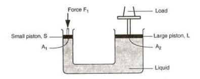
At the smaller piston S the force applied  $F_1$  cause a pressure  $P_1$  at the cross-section area  $A_1$ .
