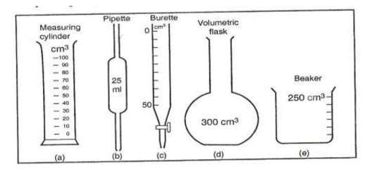
**NOTE:** The scale of the Burette begins from zero at the top and increases downwards to the maximum value e.g. a reading of 31.0ml on the burette means that volume of the liquid is [50-31] ml
