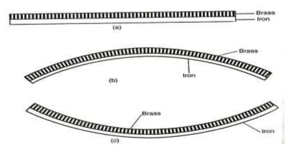
On cooling, the brass contracts more than iron. It therefore becomes shorter than the iron and thus ends up being on the inner side of the curve as shown in (c) above
