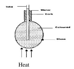
A glass flask is filled with coloured water and heated as shown above
