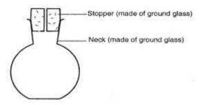
To find the density of the liquid using a density, measure the mass  $m_1$  of a dry clean density bottle with its stopper.
