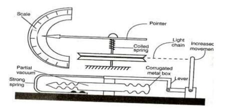
The pointer would indicate a particular value of atmospheric pressure of the surrounding so that any changes in pressure would be noticeable by movement of the pointer to either side of this atmospheric value on the scale.
