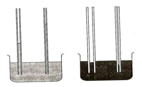
a) Glass tubes dipped in water mercury
