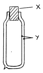
The vacuum is a double walled glass vessel with a vacuum in the space between the walls. This minimises the transfer of heat by conduction and convection. The inside of glass walls, in the vacuum side, is silvered to reduce heat losses by radiation (Poor emitter and absorber). The felt pads on the sides and at the bottom support the vessel vertically.
