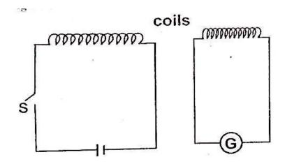
When the switch is closed, the galvanometer shows a reading and then returns to zero.
