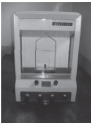
An analytical balance with an accuracy of 10^{-3} g
