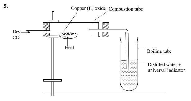
The above set-up was used to determine the chemical properties of carbon (II) oxide.
