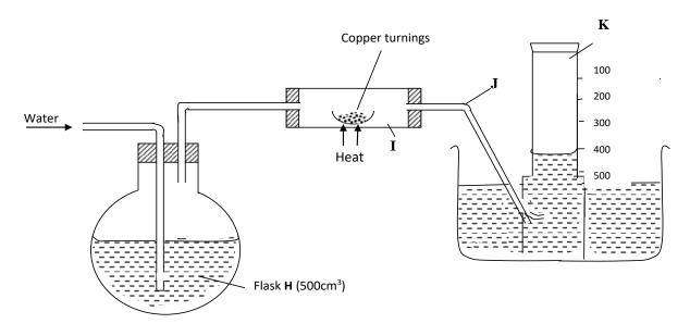
A 500cm<sup>3</sup> measuring cylinder **K** was filled with water and assembled for gas collection. Copper turnings were heated red hot and water was slowly passed into 500cm<sup>3</sup> flask **H** until it reached the 500cm<sup>3</sup> mark. A colourless gas was collected in **K**.
