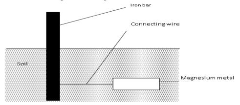
Explain why it is necessary to connect the piece of magnesium metal to the iron bar. (2mks)
