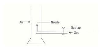
Explain how the air is drawn into the burner when the tap is opened
